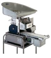
Optional 2' neoprene or wire mesh take away conveyor provides for continuous production. Equipped with a built-in digital programmable counter for accurate patty stacking.
